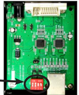
For PC, configure the switches as shown below:
